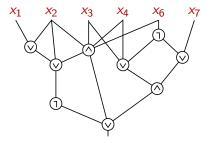
CIRCUIT SATISFIABILITY: Given a Boolean circuit C, decide if there is an assignment on the inputs of C making the output true.
