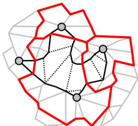
**Key idea:** the paths of the dual solution between the branch points/crossing points can be assumed to be shortest paths.
