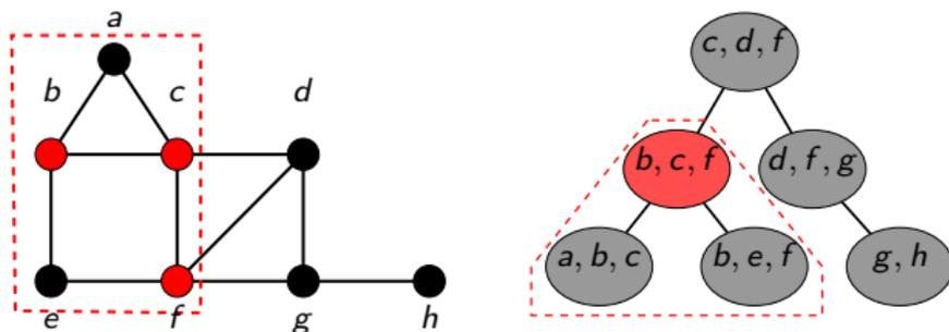
A subtree communicates with the outside world only via the root of the subtree.
