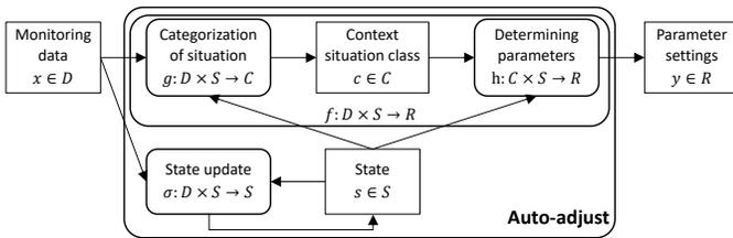
Fig. 3: Proposed structure of the Auto-adjust step
