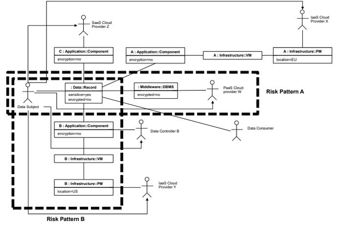
Fig. 2. Example cloud system model, in which the found risk pattern instances are marked by dashed frames [13]
