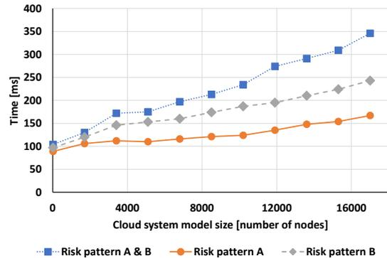
Fig. 7. Duration of pattern matching for growing cloud system models
