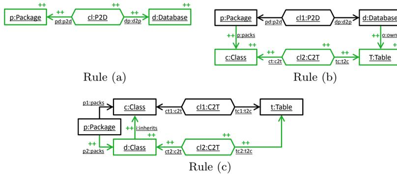
**Fig. 2.** TGG Rules (a)–(c) for the integration
