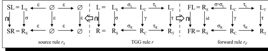
**Example.** From Rule (c) of our running example (Fig. 3), the operational rules  $r_S$  and  $r_F$  depicted in Fig. 4 can be derived. The source rule extends the source graph by adding an **Employee** to an existing **CEO** in a **Company**, while the forward rule  $r_F$  transforms an existing **Employee** of a **CEO** by creating a new **E2P** link and a **PC** in the corresponding **Network**.
