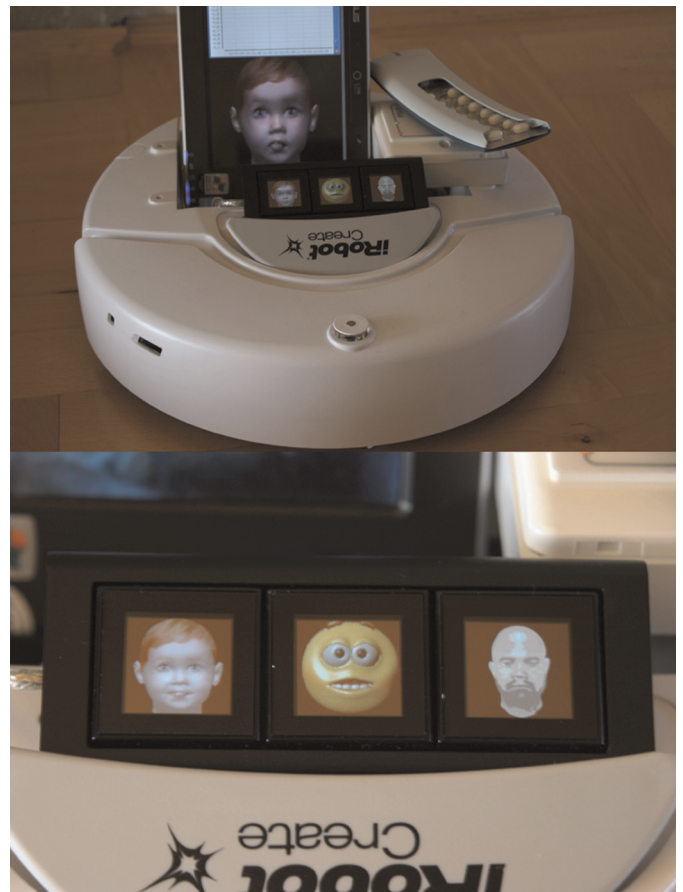
Figure 2 The ambient facial interface provides immediate visual feedback and an easy-to-understand display of compliance levels
