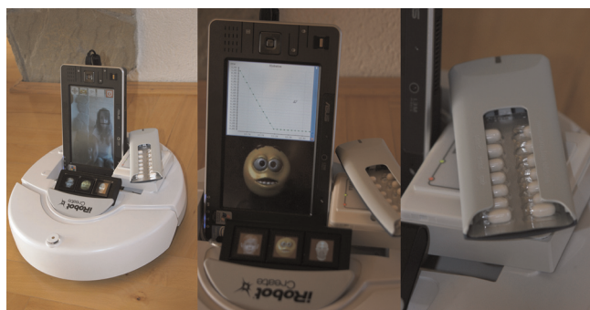
Figure 1 The home robot uses face recognition, an ambient facial interface and an intelligent pill dispenser combined with RFID technology
