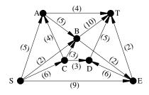
7. (MT+'18) Determine a maximum flow and a minimum s,t-cut in the network below.
